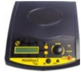
backwards in time (the Webbox will tell you what the new time position is). If you press the volume knob again, the reading will begin where you set it using the volume knob. To confirm this, you can also press the [OK] button. On the remote control, you use the [<<Left] or [>>Right] button for this. Please note: Fast forward and backwards only works within a chapter.
